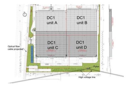
Considering the **construction footprint**, the impact of the high voltage line is however limited:
